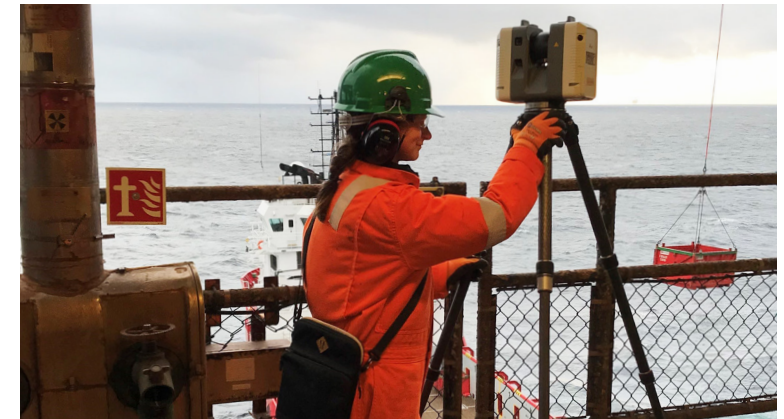
Magda Oglodek of GDi laser-scanning the Bruce Platform for the digital twin
